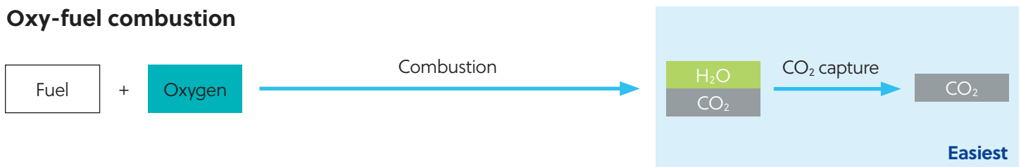
Figure 3. Material science methods: simplified schematics of CO 2 capture processes
